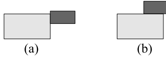
Fig. 1. Two objects in a scene touch each other. In situation (a) the objects touch on their sides no object support should be expected. Situation (b) will lead in some case to object support.
